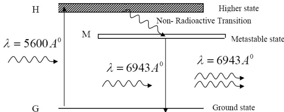
The transition between H and M is non-radioactive transition i.e. the chromium ions gives their energy to the lattice in the form of heat. In the Meta stable state the life time of chromium ions is  $10^{-3}$  sec. The life time of chromium ions in the Meta stable state is  $10^5$  times greater than the life time of chromium ions in higher state.
