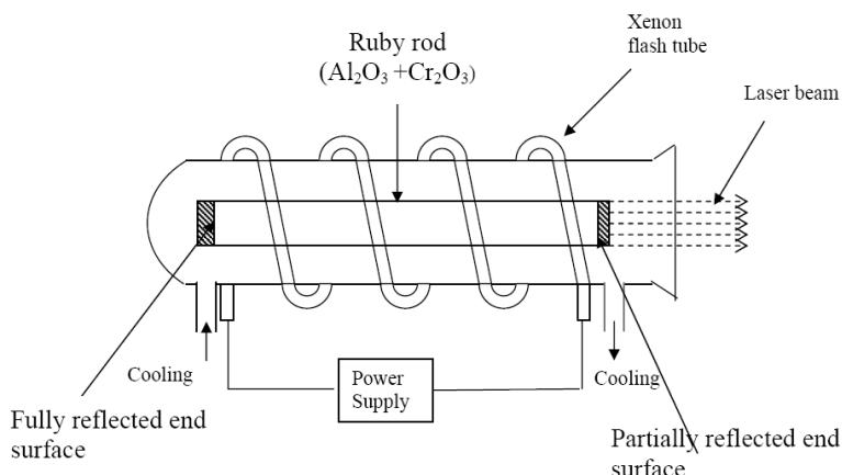
Xenon flash tube emits thousands joules of energy in few milli seconds, but only a part of that energy is utilized by the chromium ions while the rest energy heats up the apparatus. A cooling arrangement is provided to keep the experimental set up at normal temperatures
