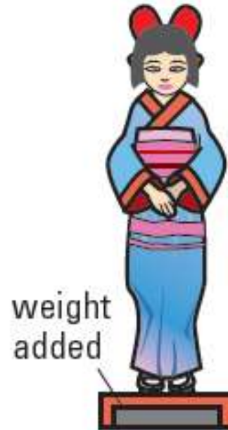
Figure 5.25c centre of gravity lowered by adding lead to base
