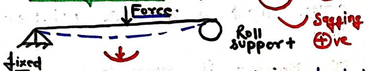
A B.M. is the reaction induced in a structural element when an external force or moment is applied to the element causing the element to bend.
