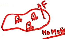
The moment of a force is a measure of its tendency to cause a body to rotate about a specific point or axis.
