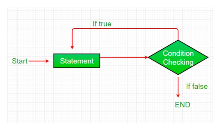
1. do while loop starts with the execution of the statement(s). There is no checking of any condition for the first time.
