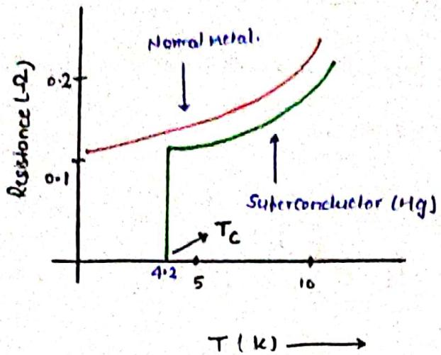
it was observed that the electrical resistance / Resistivity of Mercury decreased continuously from its melting point ( $233\text{K}$ ) to  $4.2\text{K}$  & then dropped suddenly to zero resistance. Similar results were obtained by using various other metals such as. Pb, Sn and In. Hence
