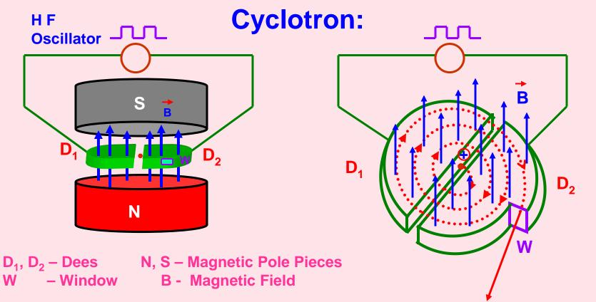
**Working:** Imagining  $D_1$  is positive and  $D_2$  is negative, the + vely charged particle kept at the centre and in the gap between the dees get accelerated towards  $D_2$ . Due to perpendicular magnetic field and according to Fleming's Left Hand Rule the charge gets deflected and describes semi-circular path.
