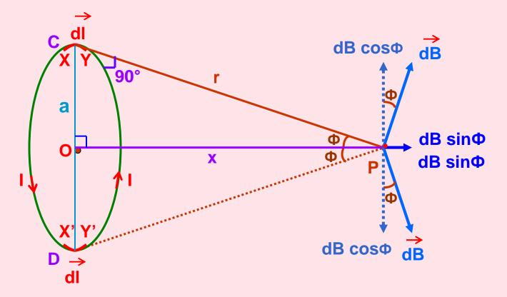
The plane of the coil is considered perpendicular to the plane of the diagram such that the direction of magnetic field can be visualized on the plane of the diagram.
