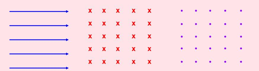
Uniform field on the plane of the diagram
