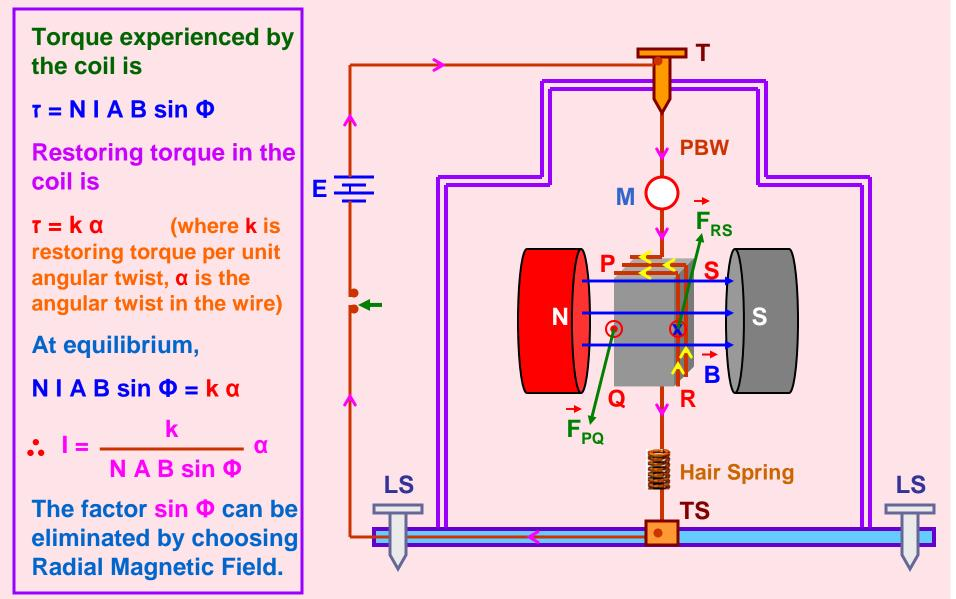
T – Torsion Head, TS – Terminal screw, M – Mirror, N,S – Poles pieces of a magnet, LS – Levelling Screws, PQRS – Rectangular coil, PBW – Phosphor Bronze Wire
