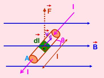
Force experienced by the electrons in dI is  $d\vec{F} = n \ A \ dI \left[ - e \left( \vec{v}_d \times \vec{B} \right) \right] = - n e \ A \ v_d \ (dI \ X \ \vec{B})$   $= I \ (dI \ x \ \vec{B})$   $\vec{F} = \int d\vec{F} = \int I \ (dI \ x \ \vec{B})$ where  $I = neAv_d$  and -ve sign represents that the direction of dI is opposite to that of  $v_d$ )
