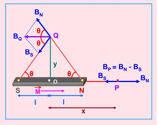
Magnetic Field at a point on the axial line acts along the dipole moment vector.
