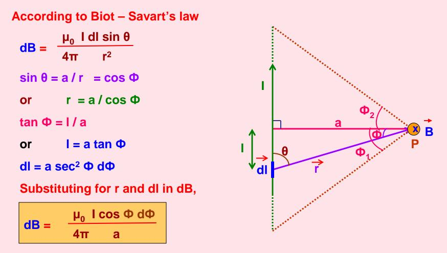
Magnetic field due to whole conductor is obtained by integrating with limits -  $\Phi_1$  to  $\Phi_2$ . ( $\Phi_1$  is taken negative since it is anticlockwise)
