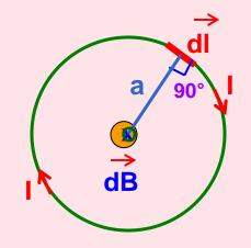
The angle  $\theta$  between dI and a is 90° because the radius of the loop is very small and since sin 90° = 1
