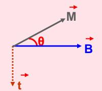
Direction of Torque is perpendicular and into the plane containing M and B.
