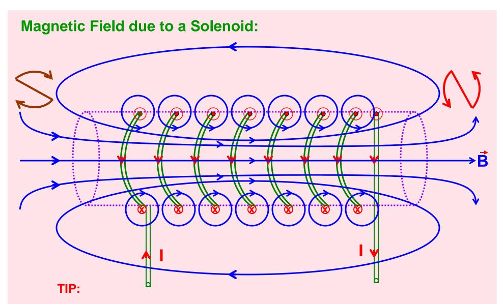
When we look at any end of the coil carrying current, if the current is in anti-clockwise direction then that end of coil behaves like North Pole and if the current is in clockwise direction then that end of the coil behaves like South Pole.
