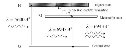
The transition between H and M is non-radioactive transition i.e. the chromium ions gives their energy to the lattice in the form of heat. In the Meta stable state the life time of chromium ions is  $10^3$  sec. The life time of chromium ions in the Meta stable state is  $10^5$  times greater than the life time of chromium ions in higher state.
